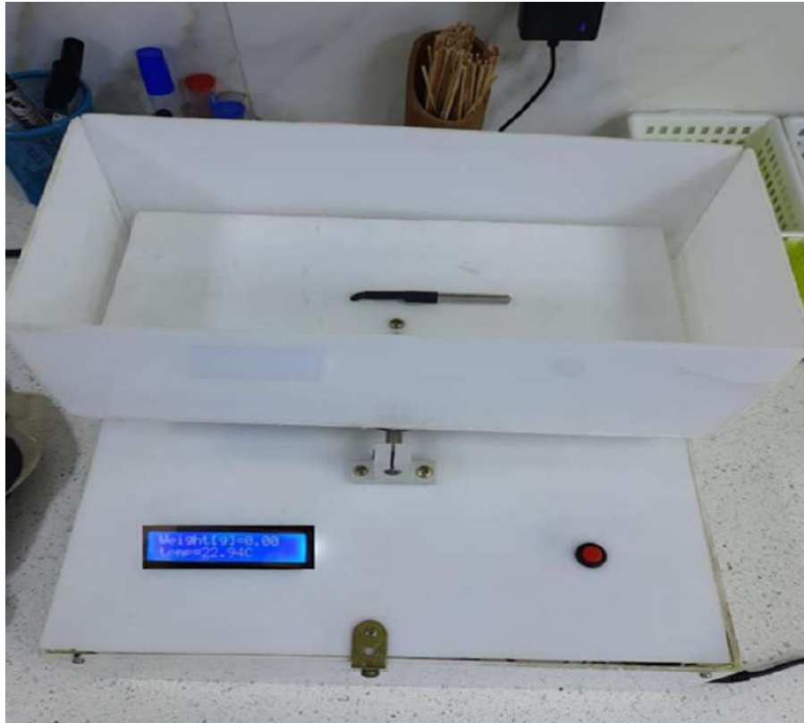
Fig (4-4). Shown Temperature and Weight After operation of the Shaking Blood Bag Device
