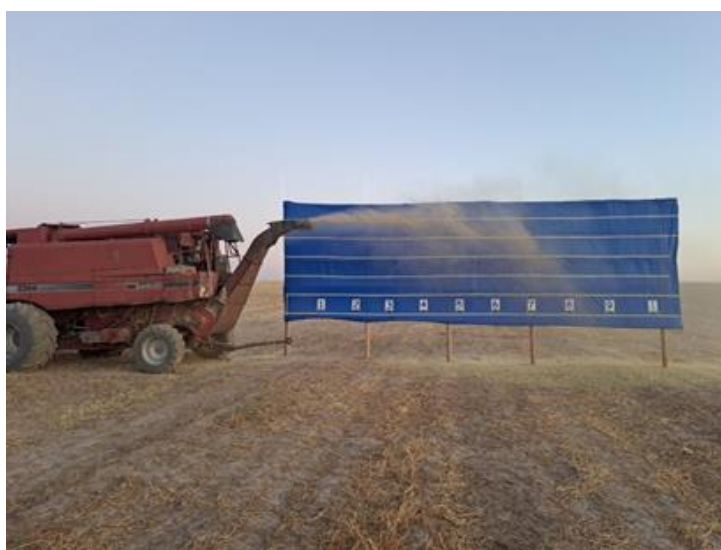
Figure 2. Effect of Number of Straw Loader Drum Blades on Straw Throwing Distance Study Process
