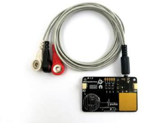
Fig 2.3 Proto Central MAX86150 with LEDS Cable
